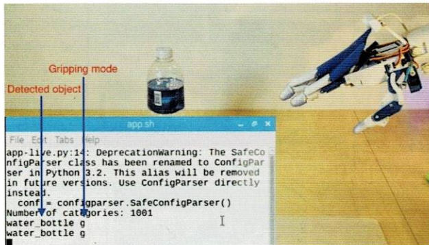
Figure 4. Hand recognizing a Pet bottle using AI program. Hand is recognizing the bottle by outputting the name of object on the first row and the second row shows the mode of gripping for the object that was detected which are g (grip), s (semi-pinch), and p (pinch).
